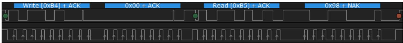
**Figure 3: I<sup>2</sup>C Read Transaction to STATUS**
