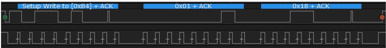
**Figure 2: I<sup>2</sup>C Write Transaction to MEAS\_MODE, 1 Second Drive Mode, Interrupts Enabled**
